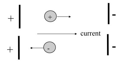
The relationship between the current I that flows between two points at potential difference  $\Delta V$  depends on the *resistance* to the flow of charge offered by the medium between the two points. This relationship can be very complicated because of microscopic processes within the medium, which in turn depends on the nature of the medium.
