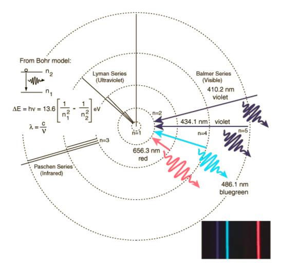
This spectrum was produced by exciting a glass tube of hydrogen gas with about 5000 volts from a transformer. It was viewed through a <u>diffraction grating</u> with 600 lines/mm. The colors cannot be expected to be accurate because of differences in display devices.
