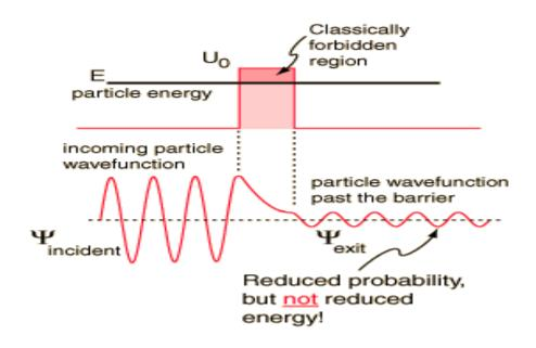
Note that having tunneled through the barrier, the particle has the *same* energy as it had before it met the barrier.
