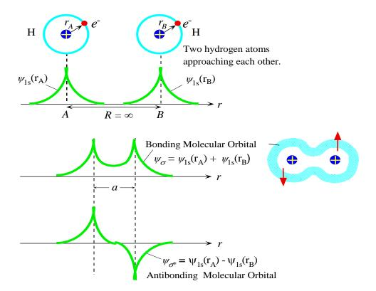
Fig. 4.1: Formation of molecular orbitals, bonding and antibonding  $(\psi_{\sigma} \text{ and } \psi_{\sigma^*})$  when two H atoms approach each other. The two electrons pair their spins and occupy the bonding orbital  $\psi_{\sigma}$ .
